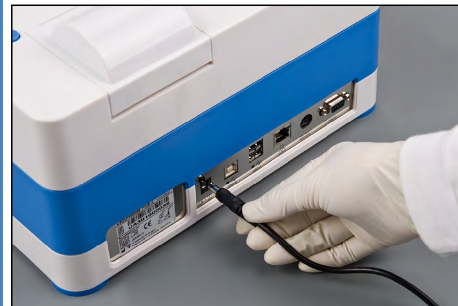
Figure 7: Plugging in the analyzer
