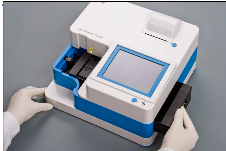
Figure 10: Inserting the test strip tray
