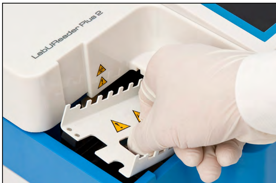
Figure 9: Inserting the strip timer rake
