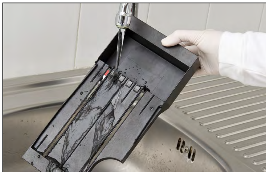
Figure 53: Rinsing the test strip tray
