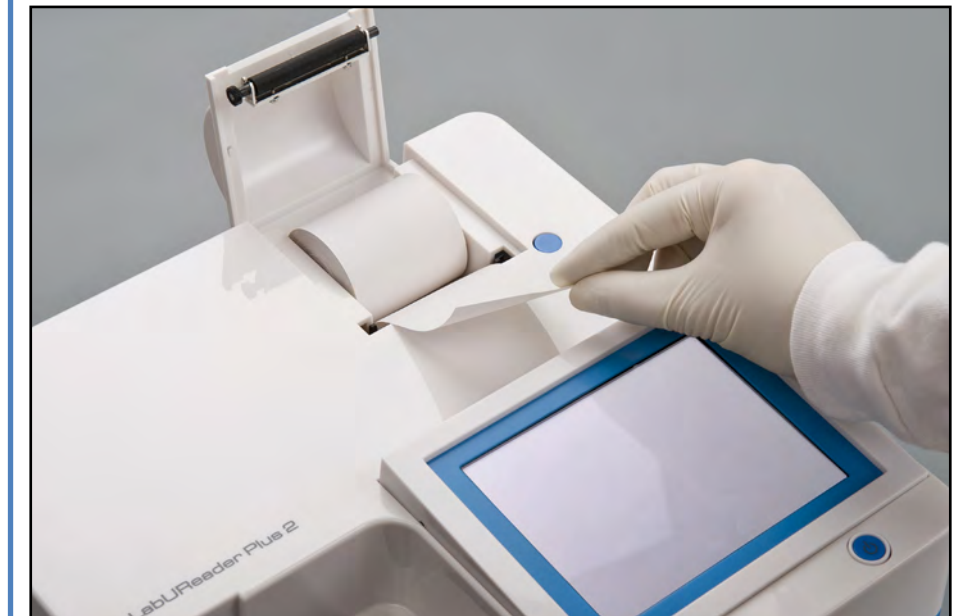
Figure 11: Loading the printer paper
