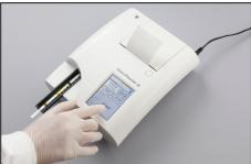
Place the reagent strip in the channel of **r** The instrument will automatically **O**detect an applied strip. The measurement cycle will be started.
