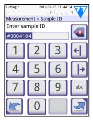
**Sample ID:** unique sampleID is assigned by default. To change it, use the onscreen keyboard, the attached keyboard or the barcode reader. Maximum 14 characters. Sample ID must not be empty.
