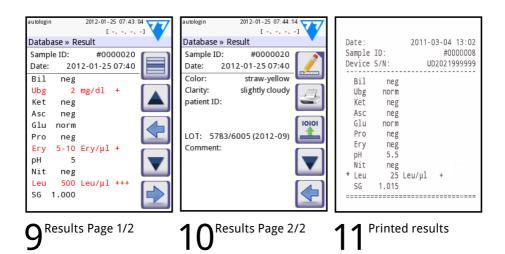
The pad results are displayed on the first page. Positive findings are clearly marked with red text on the display. To view the remaining test results, touch the **Right** icon on the screen.
