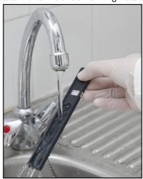
**Figure 49:** *Rinsing the test strip tray*
