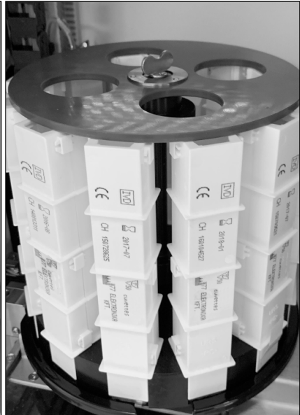
Figure 58. A fully loaded rotating cuvette carousel
