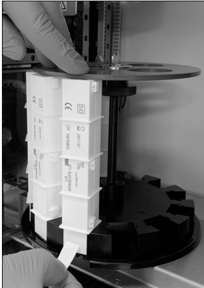
Figure 57. Loading the rotating cuvette carousel
